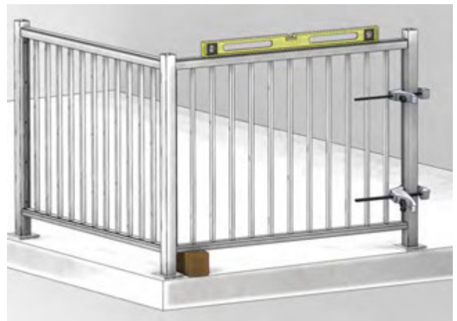
Step 3 Due to the slope in the balcony floor, you can start with a block but use a level for the railing
