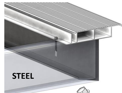
P-6 installed on Steel structure #14 2" Self drilling screw
