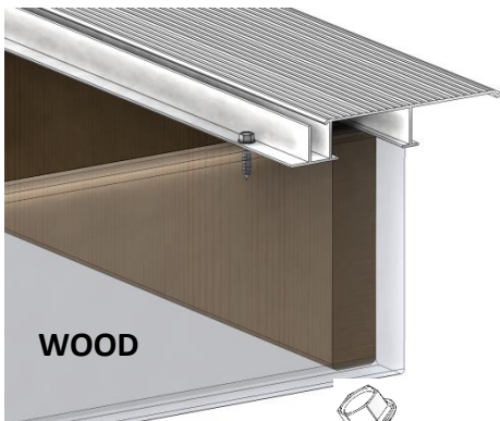
P-6 installed on Wooden structure #14 1" screw
